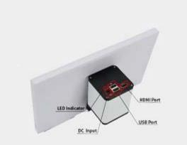
White Balance Exposure Display Frame rate Scanning method Shutter Speed Operating Temperature Magnification / Zoom Saving function Auto / Manual Auto / Manual 1080P@60fps/1080P@50fps Line by line scanning 1/50s(1/60s) \-1/10000s 0°C ~ 50°C Support Support U disk storage
